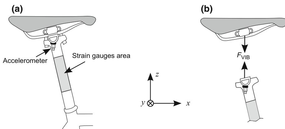
**Fig. 3** Instrumented stem
