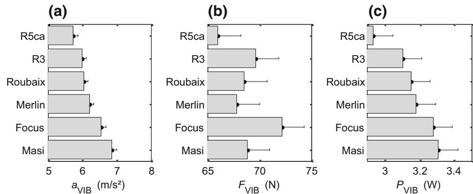
**Fig. 9** Stem VIB measurement at the right brake hood, uncertainty bars are at a confidence level of 95 %
