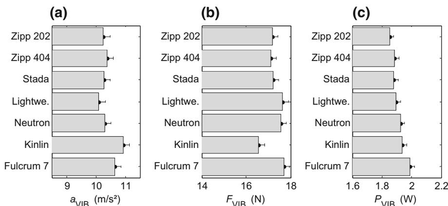
**Fig. 6** Forks VIB measurements at the left brake hood, uncertainty bars are at a confidence level of 95 %
