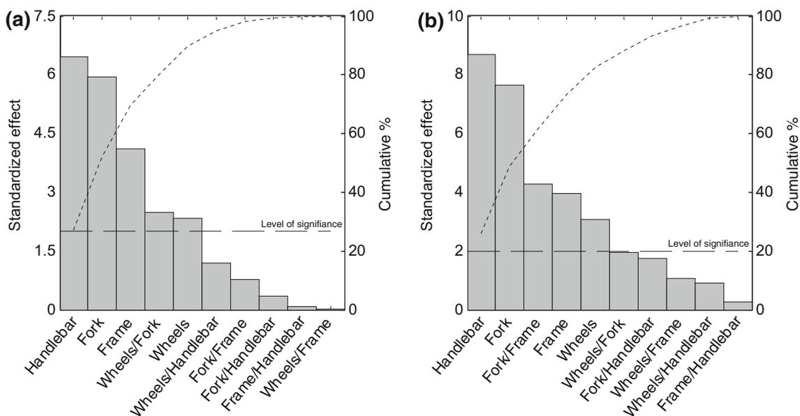
**Fig. 12** Pareto Chart, standardized effects and cumulative effects of the bicycle components on  $F_{VIB}$  **a** at the left brake hood; **b** at the right brake hood; the factors above the level of significance have a  $p$  value below 0.05
