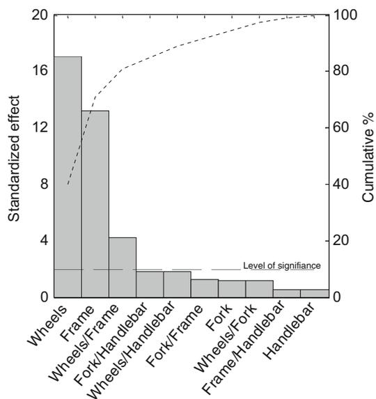
**Fig. 16** Pareto Chart, standardized effects and cumulative effects of the bicycle components on  $P_{VIB}$  at the seat post; the factors above the level of significance have a  $p$  value below 0.05
