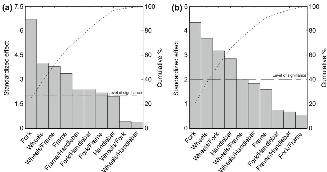
**Fig. 11** Pareto Chart, standardized effects and cumulative effects of the bicycle components on  $a_{VIB}$  **a** at the left brake hood; **b** at the right brake hood; the factors above the level of significance have a  $p$  value below 0.05
