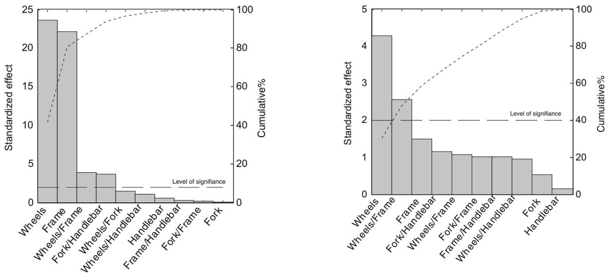
**Fig. 14** Pareto Chart, standardized effects and cumulative effects of the bicycle components on  $a_{VIB}$  at the seat post; the factors above the level of significance have a  $p$  value below 0.05
