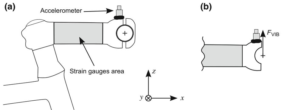
**Fig. 4** Instrumented brake
