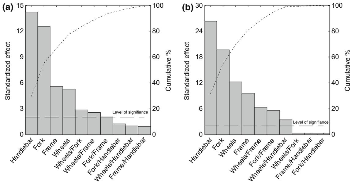
**Fig. 13** Pareto Chart, standardized effects and cumulative effects of the bicycle components on  $P_{VIB}$  **a** at the left brake hood; **b** at the right brake hood; the factors above the level of significance have a  $p$  value below 0.05
