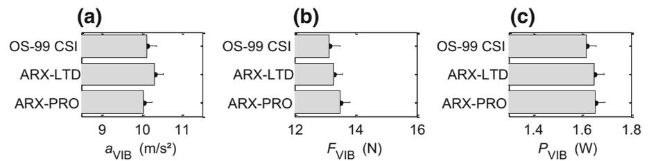
**Fig. 10** Handlebar VIB measurements at the right brake hood, uncertainty bars are at a confidence level of 95 %
