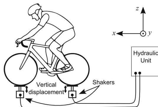
Fig. 1 Bicycle excitation setup: the road simulator
