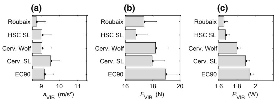
**Fig. 7** Frames VIB measurements at the stem, uncertainty bars are at a confidence level of 95 %
